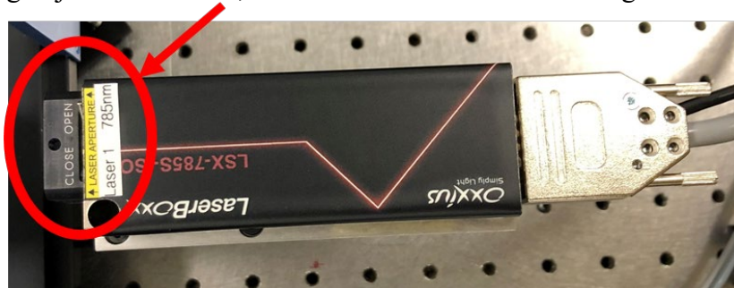
Oxxius 785nm laser Zoom in of the laser aperture switch.
