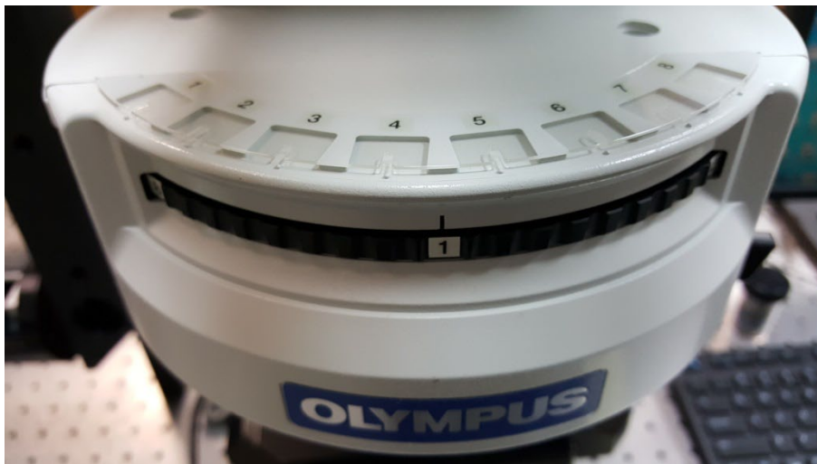
Figure 2: Filter cube selection wheel. Setting 1 corresponds to spectroscopy mode. Setting 2 corresponds to bright field viewing mode.
