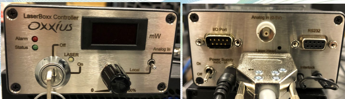
Oxxius 532nm laser system controller. (left) Front view. The key switch should always remain inside of the Oxxius box for safekeeping. (right) Back view. To turn on the controller, flip the “On/Off” switch to the “On” position.
