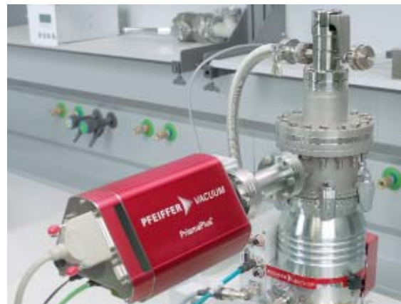
Residual gas analysis with HiPace™ and PrismaPlus™
