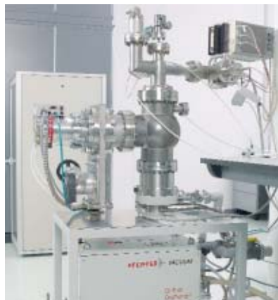
Calibrating pumping station with HiPace™ and OnTool DryPump™
