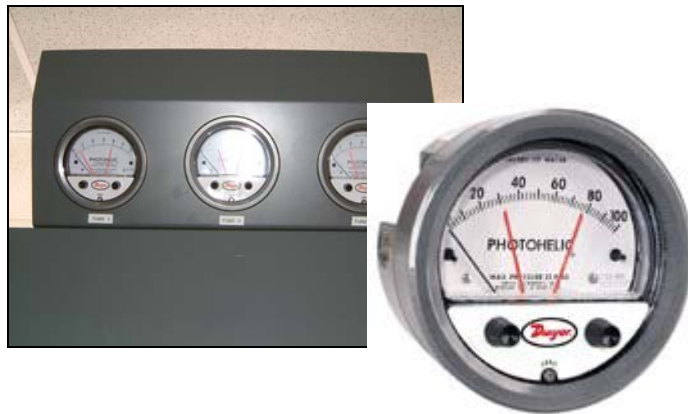
Figure 2-7 Photohelic with high and low alarm limits
