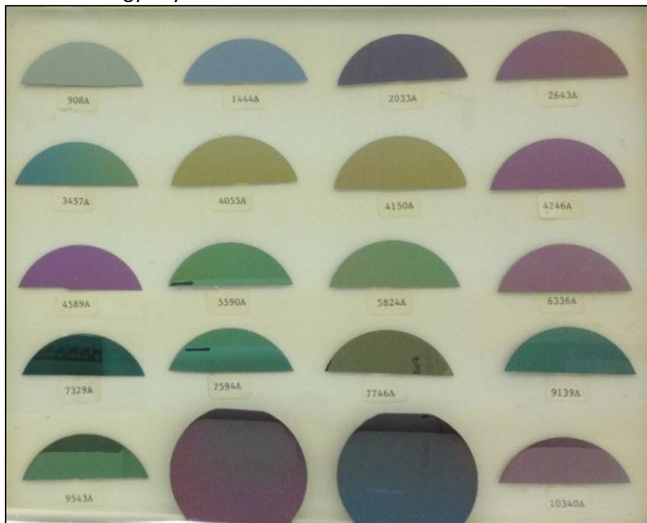
Figure 10 – Wafer Oxide Thickness Color Guide
