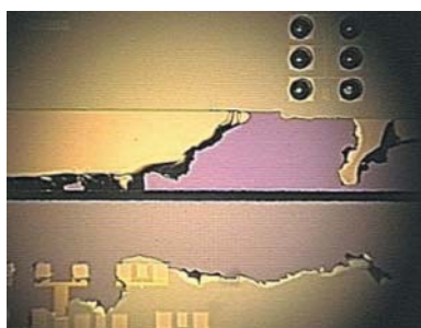
Low-k layer delamination resulting from the use of a standard blade.
