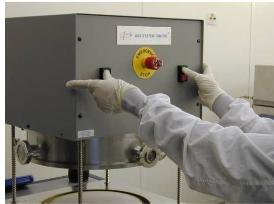
Fig. 4- Push & hold green buttons to open chamber
